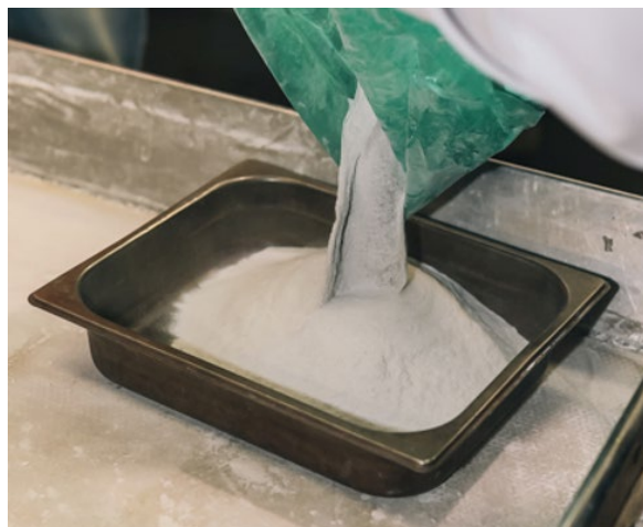
Figure 1 – Typical 6% Spodumene Concentrate from Kathleen Valley.
